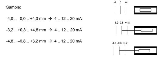
Adjustment with the zero trimmer has no effect on the gain setting. Adjustment with the gain trimmer has small effect on the zero setting.
